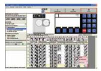
washers geographic location. IMTx also allows users to reverse the process by uploading a single machine's programming parameters onto a smart card. That information can then be used to program other machines, or it can be downloaded onto the IMTx and e-mailed to another account. Finally, the IMTx also features a programming simulator, perfect for control operation training with staff.
